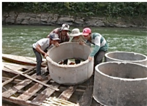
Fig. 12 – Newly cast concrete cement rings used for aquaculture, specifically fish-raising
